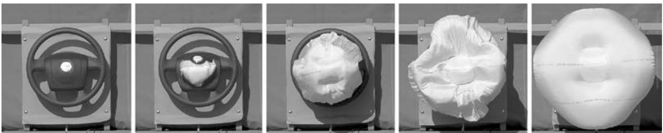
Different images of a highspeed sequence of an airbag inflation, which was recorded with two highspeed cameras. With the stereo setup it was possible to analyze the airbag inflation in three dimensions without any marker on the airbag.
