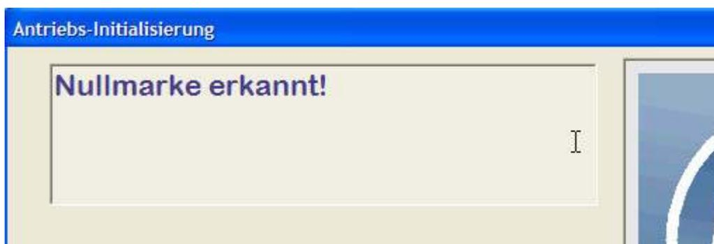
The switching on procedure and initialisation is now finished. This needs not to be done before every calibration, only once a day is normally sufficient.
