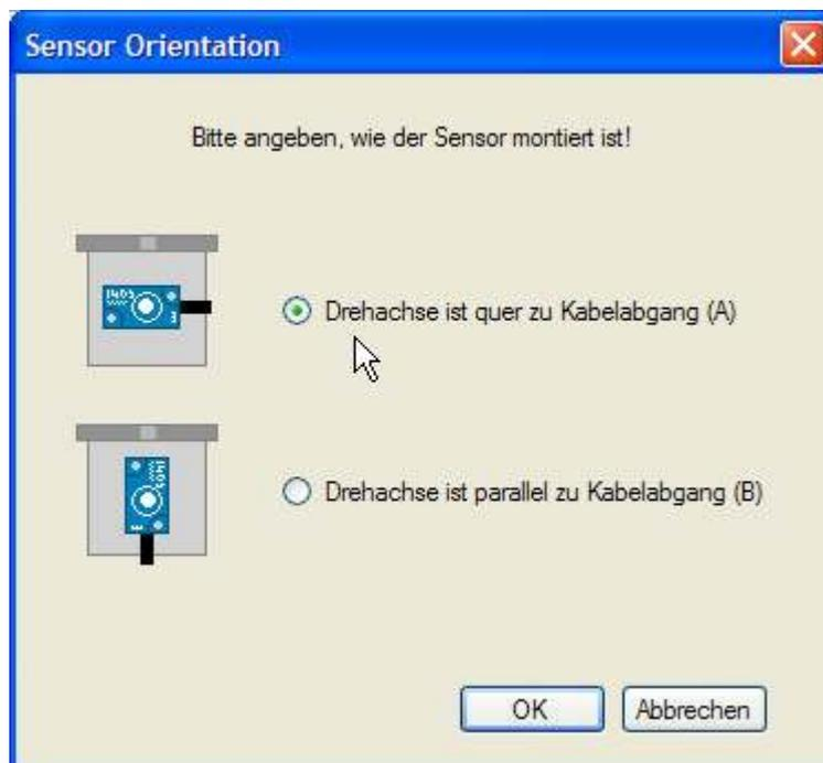
After this selection is done and OK was given, the dialog is closed, and in the main window the START button is enabled. Before starting, it is now possible to check or uncheck the box "Cal headover". The software proposes this from the data of the sensor TEDS, but it can be changed at this time. If user uses a headover mounting in her/his application, the calibration should also be performed headover, so normally the suggestion should not be touched.
