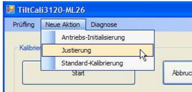
At this point the sensors electronic data sheet TEDS is read and its serial number is cross checked with the logged in DUTs. All data from this sensor lands in the already created result file named after the sensors serial number. It is a good practice to remove the result files to another directory, after the calibration job is done.
