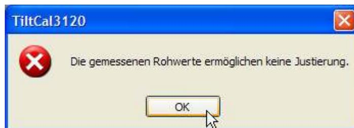
Possible sources of errors are, that the sensor was not mounted to the tilt table, or was mounted with incorrect axis orientation.
