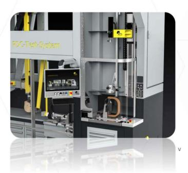
An automated drop-height positioning and quick-lock mechanism for an easy adaption and release of the head offer maximum convenience during the preparation and performance of the test. Through its design concept, the head drop test can be used for a wide range of other applications such as the rib drop test and the calibration of seat belt load cells, displacement sensors, etc.
