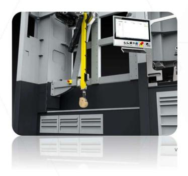
The neck pendulum offers an innovative adaption system to change the head forms quickly and easily. Also available is the neck pendulum electrical acceleration extension which provides accurate drive of the pendulum with a servo drive to reduce the required test bench height.
