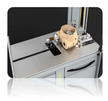
The ergonomic height of operation and the additional module of an integrated crane to conveniently move and deploy the dummy offer an efficient and simple testing process.
