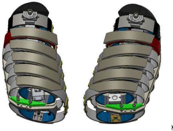
Figure 44. Mass blocks #60416 installed at bottom of thorax
