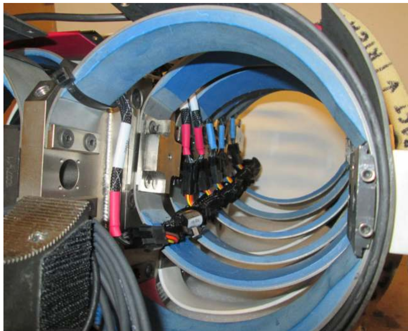
Figure 39. LED breakout cable – view from head with LED cables plugged in
