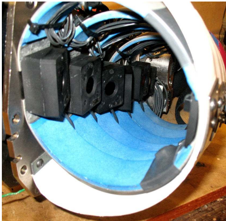
Figure 1. RibEye sensors mounted in the dummy (view from pelvis upward)
