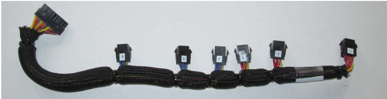
Figure 37. LED cables plugged into #70030 breakout cable
