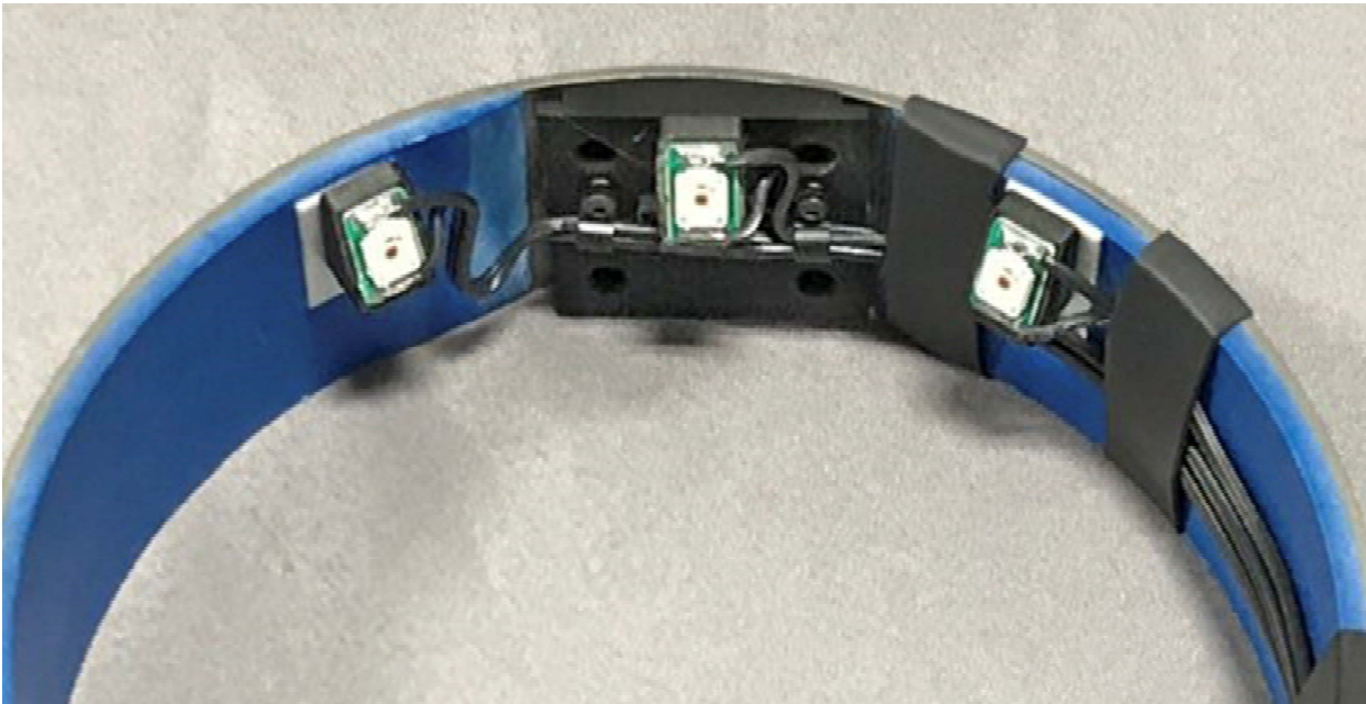
Figure 21. Alternative mounting of rearward and forward LEDs
