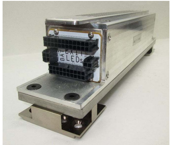
Figure 5. Controller connectors for LED breakout cable, status cable, battery cable, and dummy exit cable
