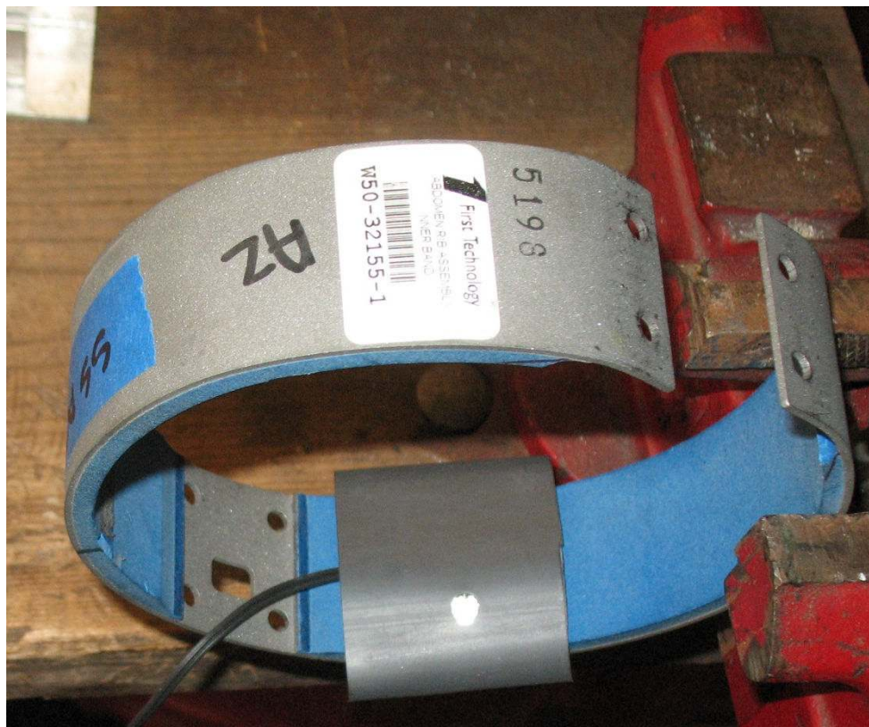
Figure 19. Heat-shrink tubing placed over rearward LED
