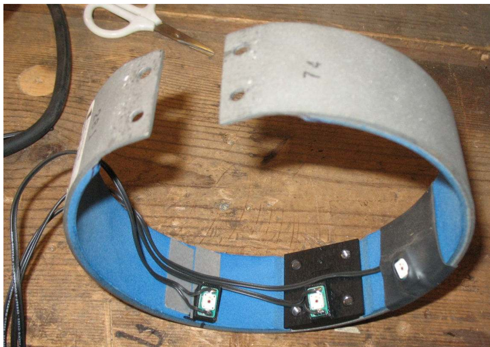
Figure 20. Cable routing for rearward and center LEDs
