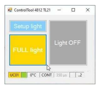
The software control panel is mostly self explaining. Setup light, full light and light off are the same as the short press of the MODE button.
