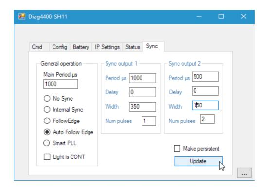
Remark: The small controller 4415 supports only one sync phase and has no internal sync generator (no PLL). It is always operated in FollowEdge mode.
