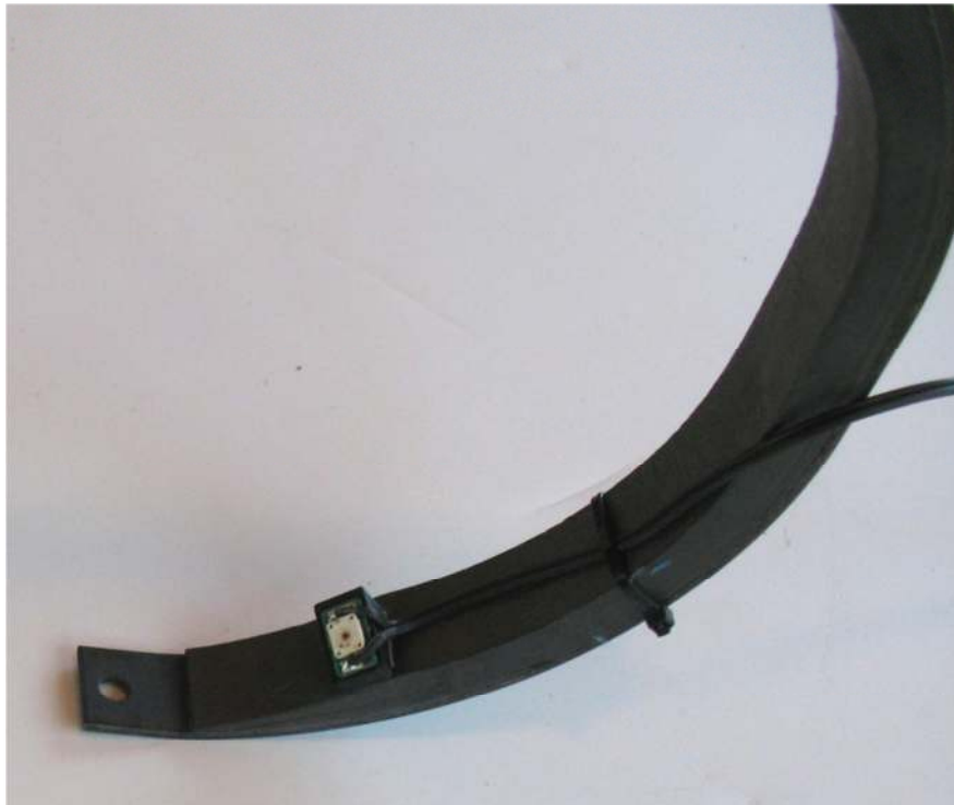
Figure 19. Angled LED in place on rib with lead wire secured by nylon tie
