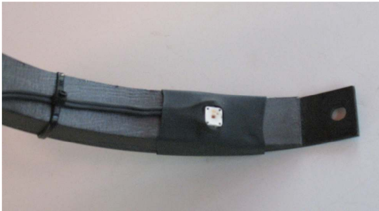
Figure 23. Flat LED in place after heat-shrinking
