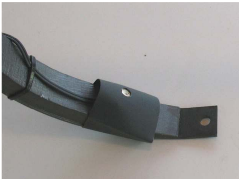
Figure 20. Heat-shrink sleeve in place over flat LED
