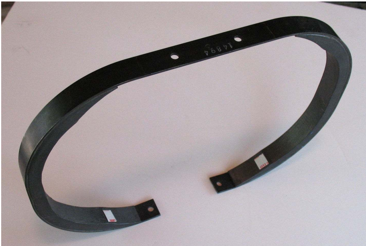
Figure 15. Rib with double-stick foam tape in place
