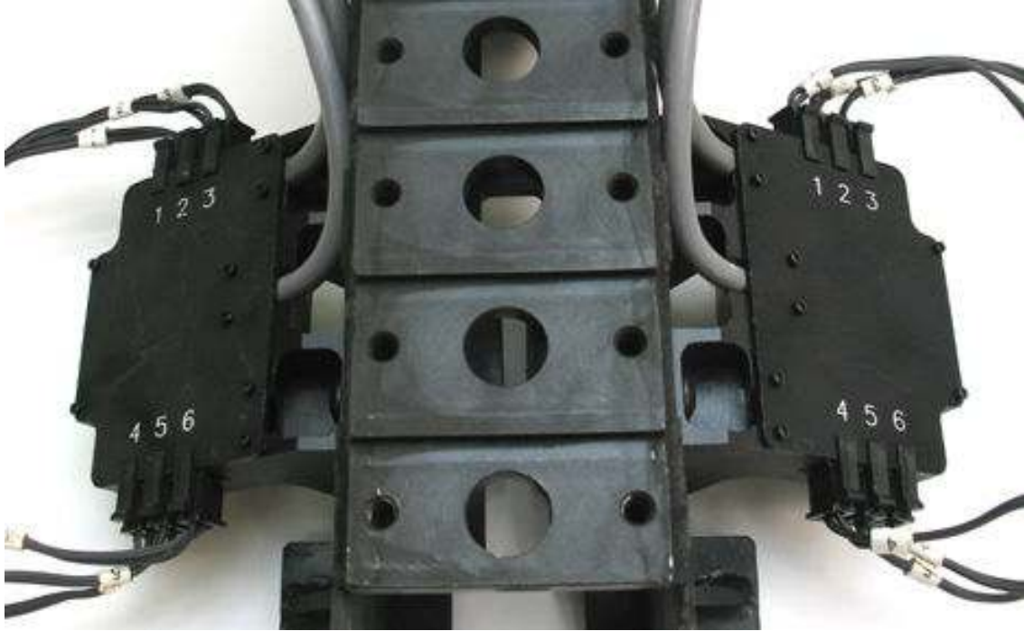
Figure B8. LED cables (lead wires) attached to connector blocks in RibEye sensor heads (rear spine view)
