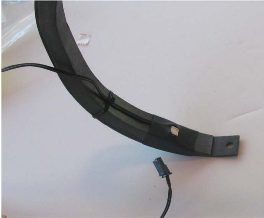
Figure 25. Flat LED and lead wire installed
