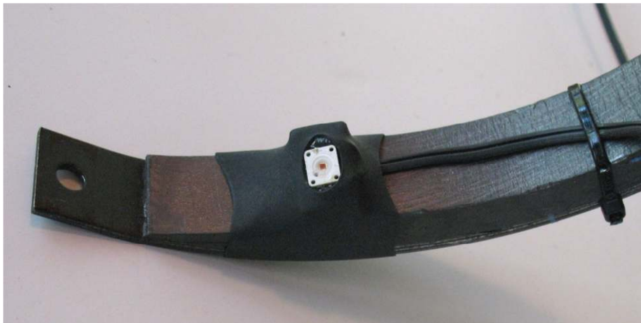
Figure 24. Angled LED in place after heat-shrinking
