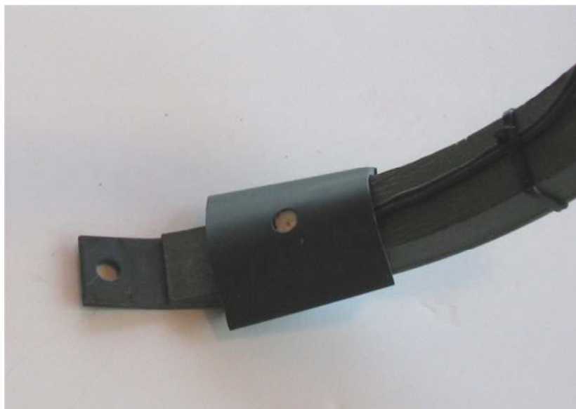
Figure 21. Heat-shrink sleeve in place over angled LED
